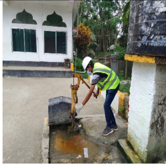
Collection of sample for Ground Water Quality Test: Chowmuhoni Poursava
